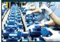
Water Pump Assembly Line
