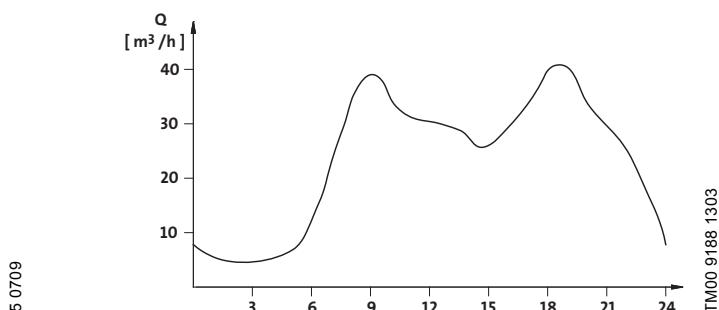
Fig. 35 Example of 24-hour consumption profile
