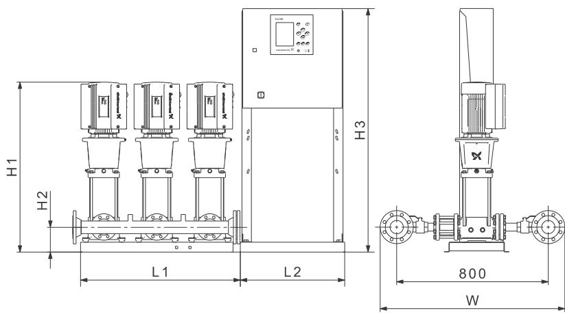
**Fig. 60** Dimensional sketch of a booster system with a control cabinet mounted on a separate base frame (design H). The booster system is shown as an example. The pumps supplied may differ from the sketch.
