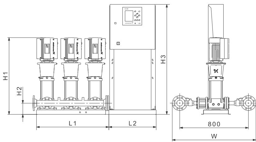
**Fig. 43** Dimensional sketch of a booster system with a control cabinet mounted on a separate base frame (design H). The booster system is shown as an example. The pumps supplied may differ from the sketch.
