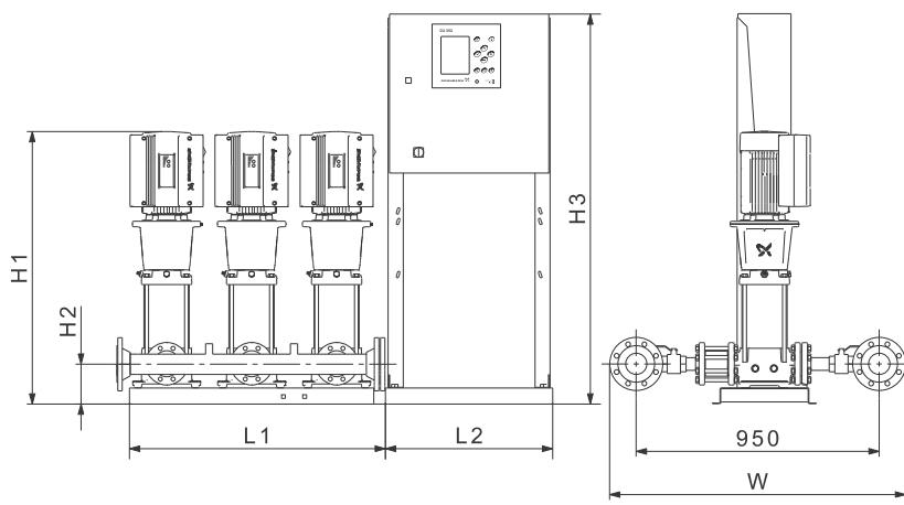
**Fig. 47** Dimensional sketch of a booster system with a control cabinet mounted on a separate base frame (design H). The booster system is shown as an example. The pumps supplied may differ from the sketch.
