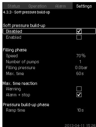
**Fig. 29** Soft pressure build-up
