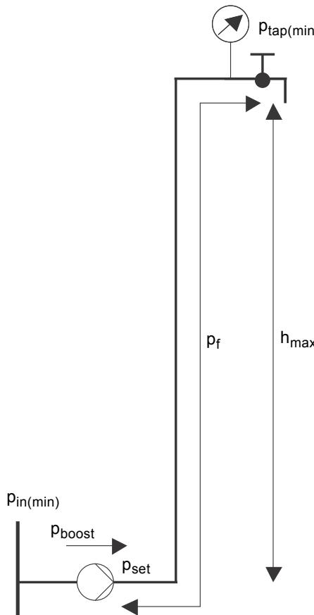
Fig. 34 Calculation of required discharge pressure
