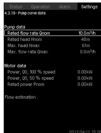
**Fig. 14** Pump curve data
